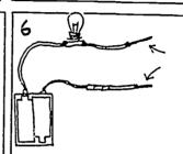
Tin the ends of the wires with a soldering iron.
